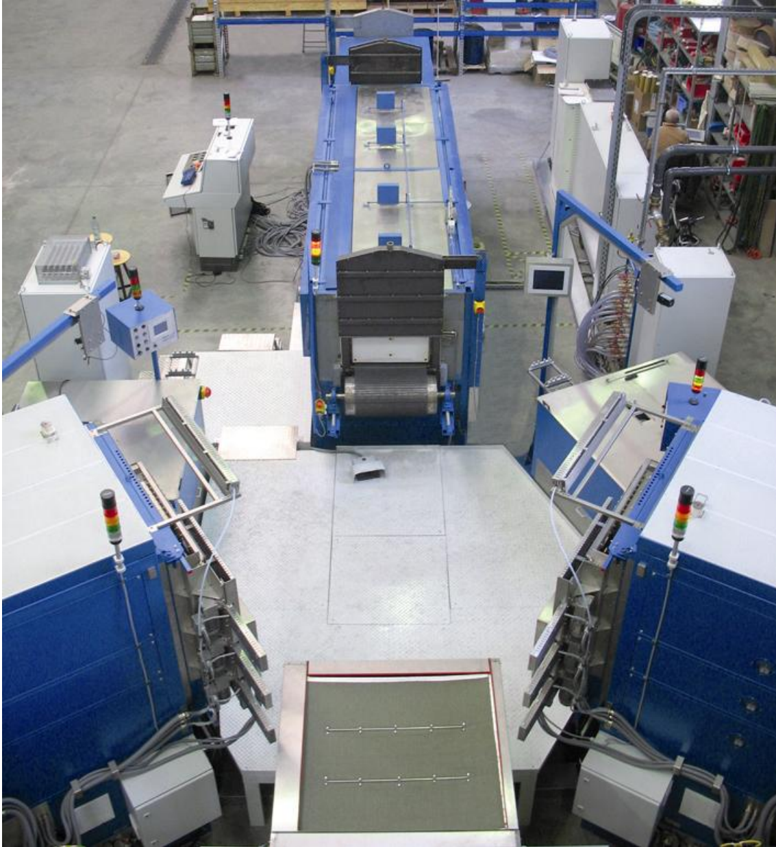
Picture 5: Automatic casting line for Titanium- and TiAl components
