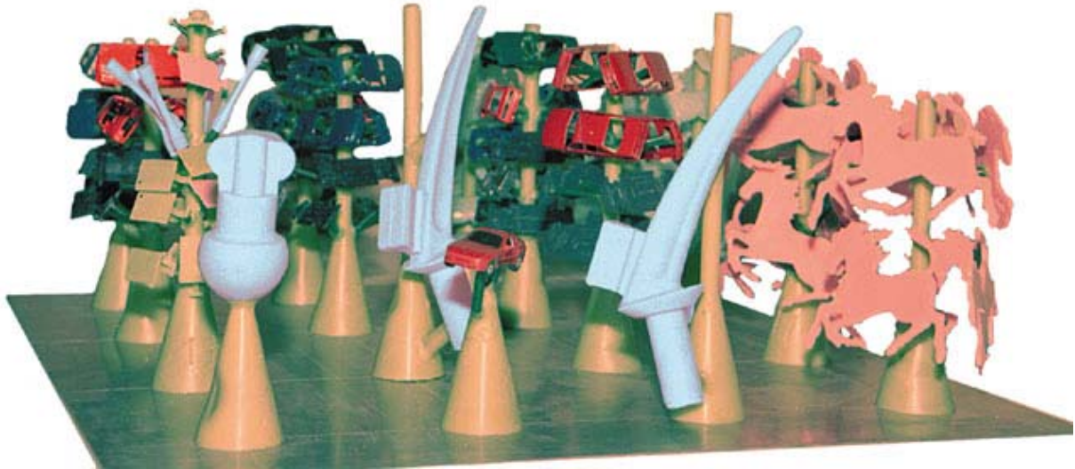
Picture 8: Wax patterns assembled to trees
