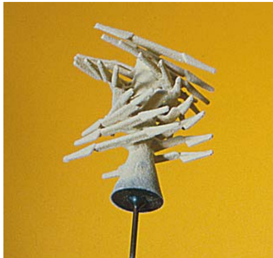
Picture 9: Pattern cluster (tree) after several sanding steps
