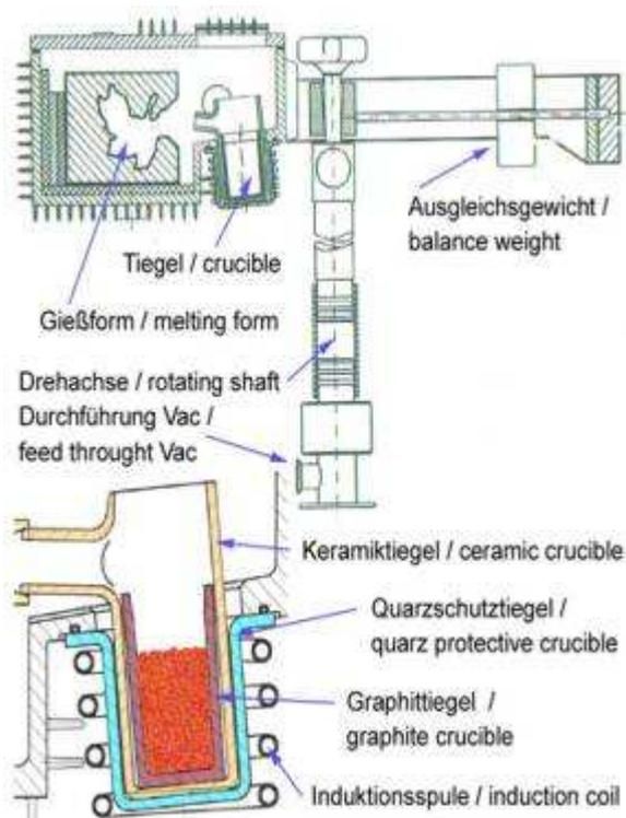
The up to date process for this is the induction heating with high or medium frequency in combination with centrifugal casting. The casting procedure is taken out as follow:
