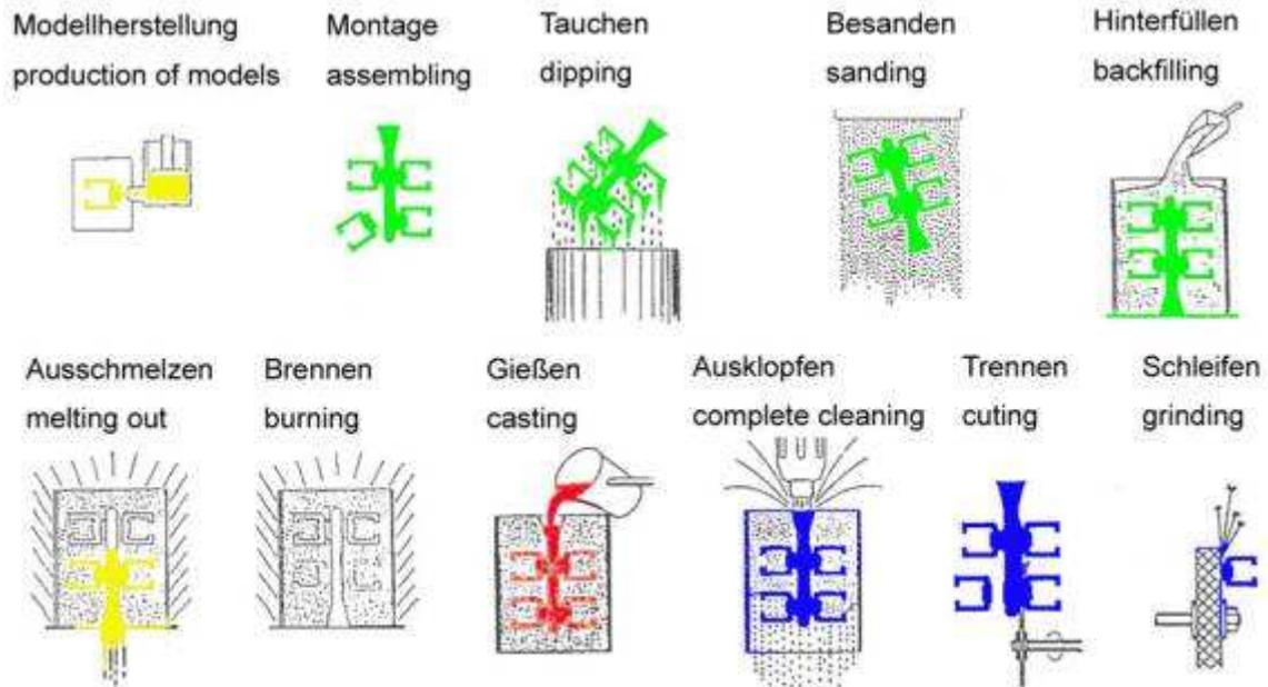
The original model, for example made of metal, will be moulded in silicone or rubber. This original mould is reproducible by filling with wax or plastic. Then the parts will be mounted in treeform and the wax model is backfilled with ceramic mass in a moulding ring made of heat-resisting steel. Depending on the material tube slurry the mould will be preheated and fit into the casting machine to fill in the metal.
