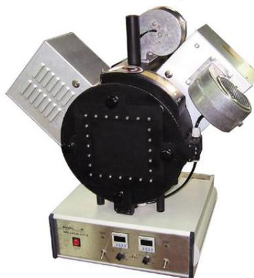
Figure 2: Dual-Frequency Laboratory Furnace (800 W 2.45 GHz / 500 W 5.8 GHz )
