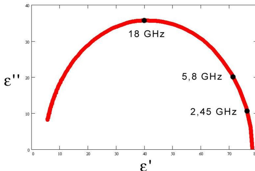
Diagram 1: Cole-Cole equation for water at 25 °C.
