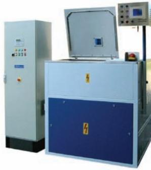
*Supercast. Induction centrifugal casting machine*
