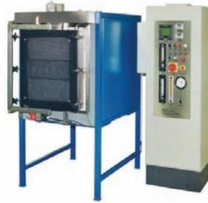
*KS-S 240 (Tmax 1200°C). Protective gas and vacuum tight, different sizes*
