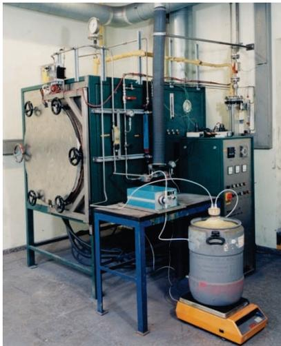
*Special furnace for catalytic debinding ( $T_{max}$  180 °C), 800l*
