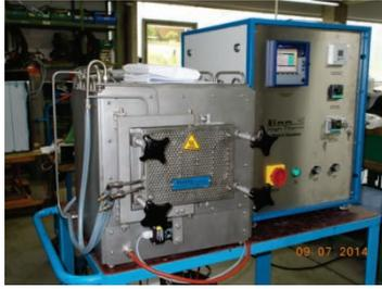
*VMK-135-S (Tmax 1050 °C). Protective gas and vacuum tight, different sizes*
