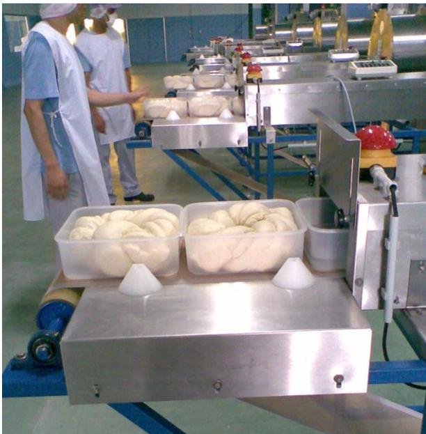
Pic. 2: Continuous Microwave Baking Ovens (Linn High Therm GmbH Model MDBT 12)
