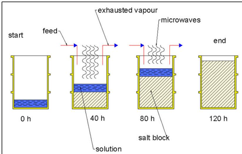
Fig. 2: Schematical construction of the MIDD Process
