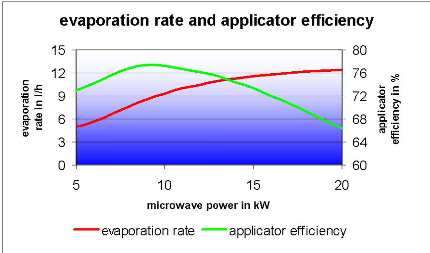
Fig. 5: Evaporation rate and applicator efficiency
