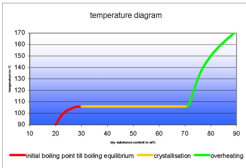
Fig. 3: Temperature diagram during the MIDD process
