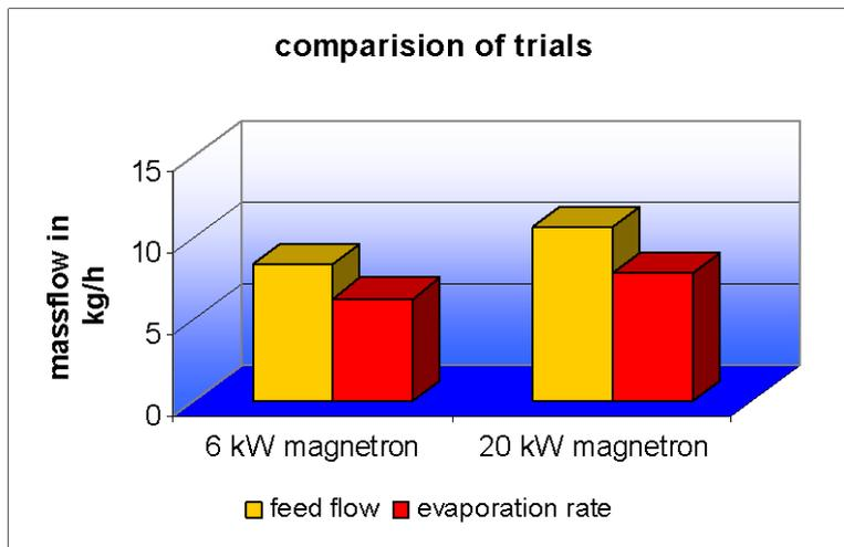
Fig. 4: Comparison of test runs with different microwave powers
