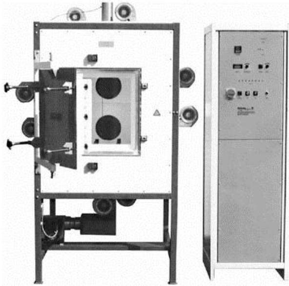
Picture 3: microwave hybrid debinding furnace 6,4 kW / 550 °C
