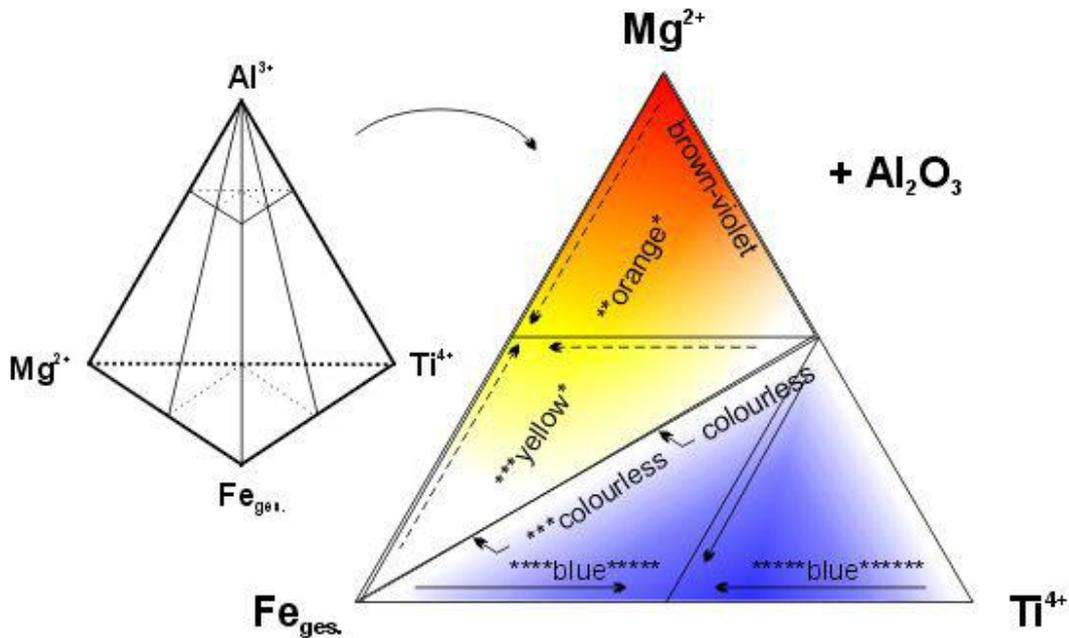
\* Defect center by Mg ± segregation of spinel
