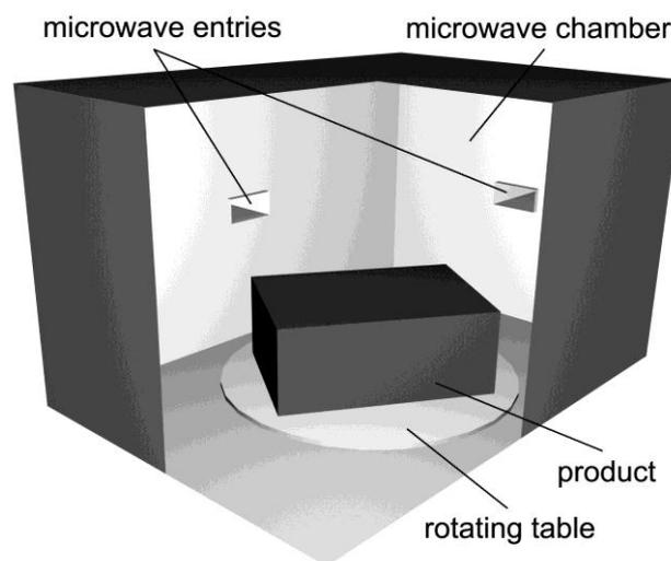
Picture 3: Multi Mode microwave chamber with rotating table
