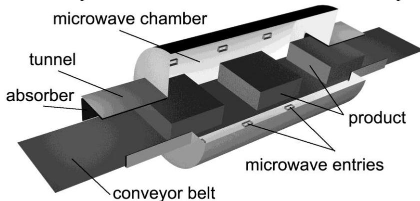
Picture 5: Microwave Multi Mode continuous belt unit
