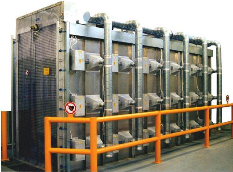
Picture 8: Microwave chamber dryer for drying of ceramic grinding wheels (Picture Linn High Therm)
