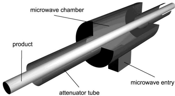
Picture 6: Single Mode  $TM_{01}$  continuous operation unit
