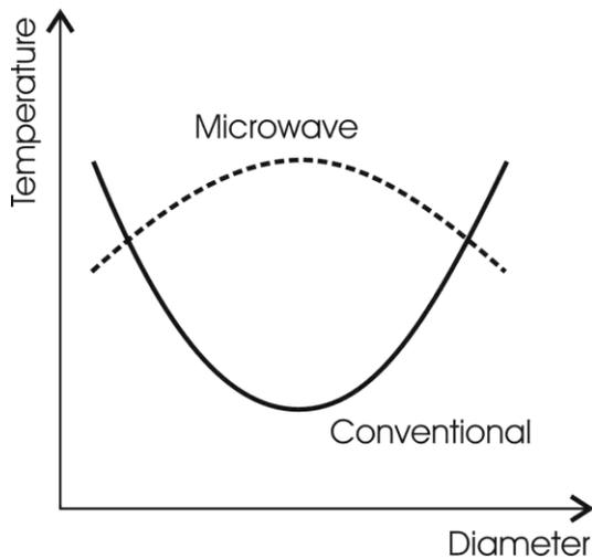
Picture 1: Temperature profile for conventional and dielectric heating
