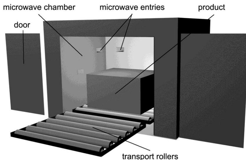
Picture 4: Microwave Multi Mode batch unit for large products
