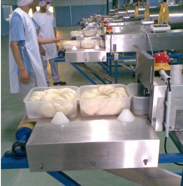
Pic. 1: Continuous Microwave Baking Ovens (Linn High Therm GmbH Model MDBT 12)
