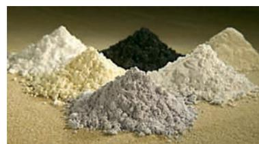
Fig. 1 RE oxides obtained after calcination: clockwise direction starting with black: Pr, Ce, La, Nd, Sm, and Gd [5]
