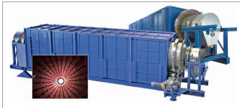
**Fig. 3 Rotary tube furnaces for monazite drying (FDHK-5-1400/10800/450, front) and digestion (FDHK-5-1800/10800/550, back); insert: paddles installed at the rotary tube interior to enhance material tumbling during processing**
