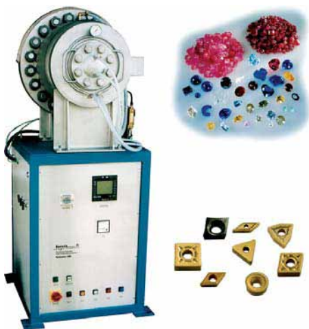
Fig. 5: High pressure furnace, "Rubistar 100", made by Linn High Therm GmbH on the left; upper right: treated corundums, like rubies and sapphires (Corundum Mine Co. Ltd., Bangkok); lower right: hard metal cutting devices (Boehlerit)
