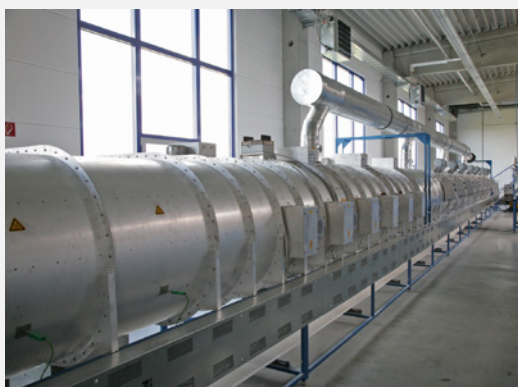
Fig. 1: Microwave belt drier MDBT 70+24/1040/210/16300, (installed Microwave power 70 kW, hot air power 24 kW, throughput approx. 2,000 – 3,000 kg/h)
