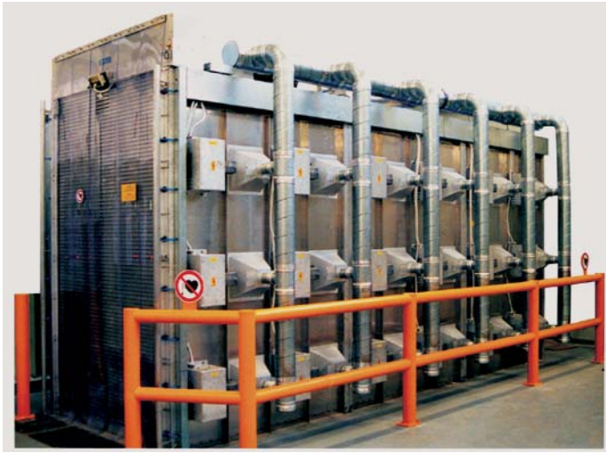
Fig. 2: Microwave chamber drier 21 m 3 / 30 kW
