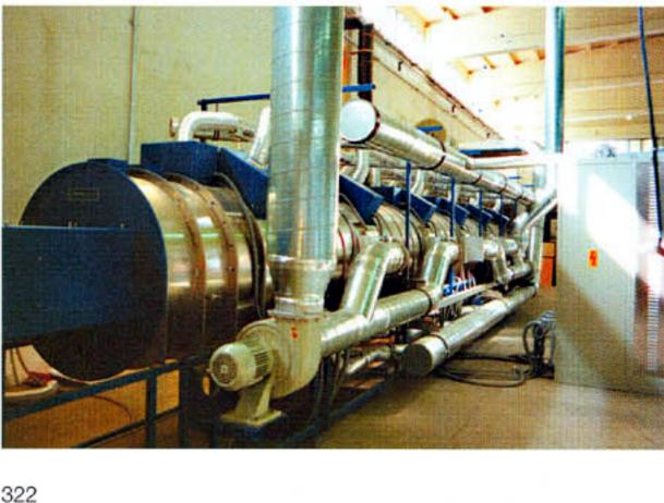
Microwave continuous belt furnace. Microwave power 60 kW, length
