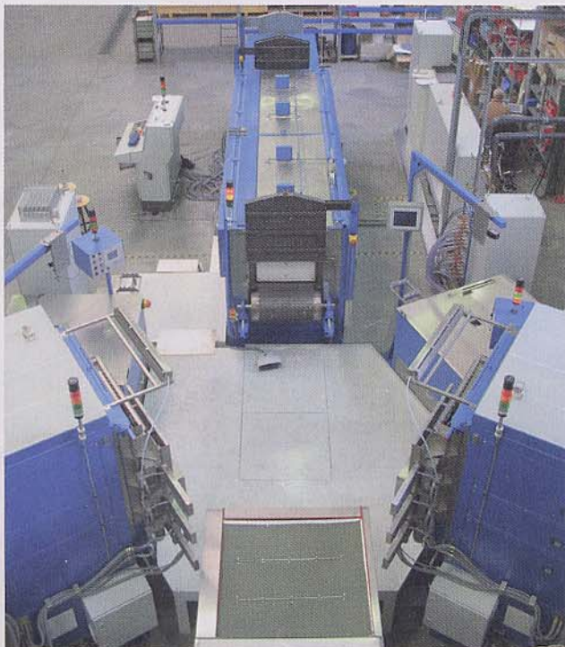
Fig. 5. Automatic casting line for titanium and TiAl components
