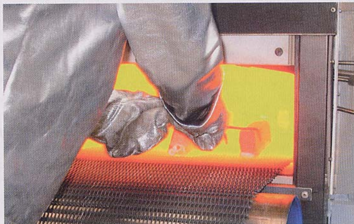
Fig. 9. Cast mold inserted into a belt heat-treat furnace
