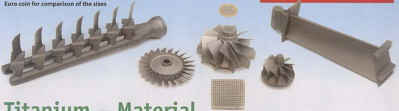
Fig. 1. Turbine blades, a casting test grid and turbocharger wheels made of TiAl with a one Euro coin for comparison of the sizes
