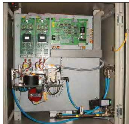
Fig. 2: Inside of 10 kW induction heating converter
