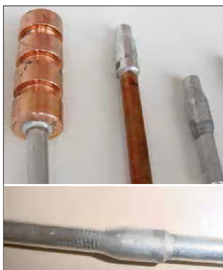
Fig. 8: Brazing with different materials (Cu/Al), Al/Al) by induction heating
