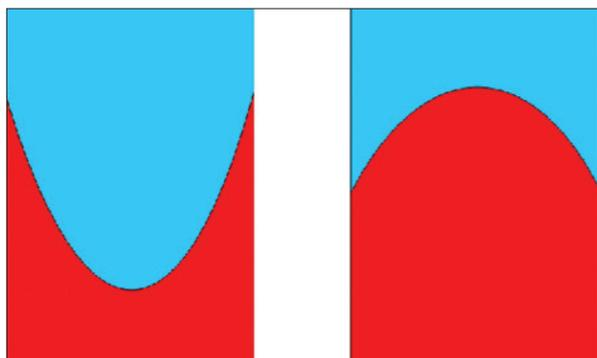
Fig. 2 Inverse temperature profile (right) of microwave technology
