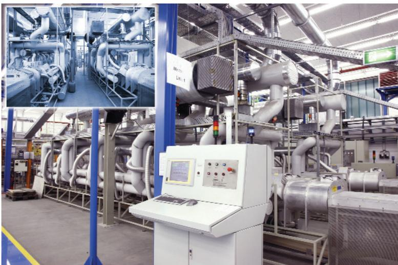
**Fig. 4** Continuous microwave belt dryer (50 kW / 20 m)
