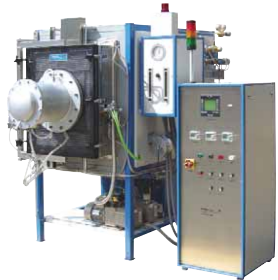
Ceramics and metal heat treatment, brazing, hardening, annealing, sintering, and debinding in atmosphere, protective gas, or vacuum. Systems for batch or continuous operation.
