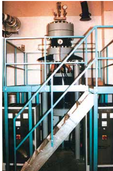
New materials 2300 °C / 200 bar Erlangen University, 1995 Most expensive furnace!
