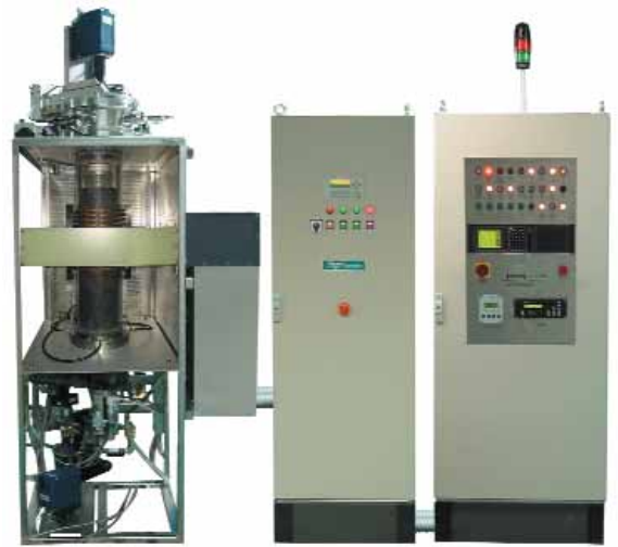
Production system for the growth of 2" SiC single crystals, 2000 The Future!
